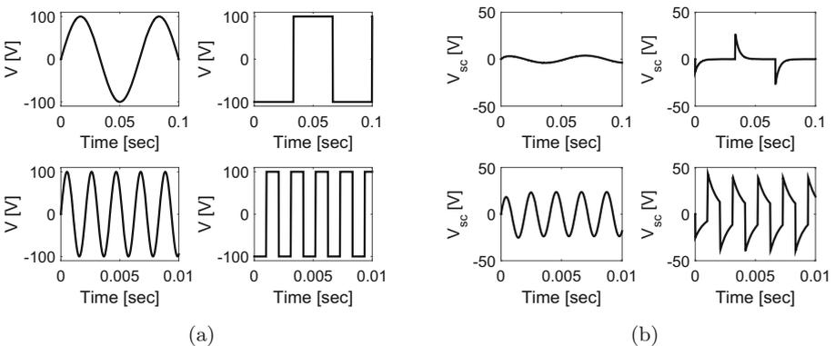
**Fig. 3.** a. The input voltage signals used in Matlab/Simulink simulations; sinusoidal and square signals at 15 Hz (first row) and 480 Hz (second row). b. The resulting voltage on the stratum corneum,  $V_{sc}$ , for the four cases.
