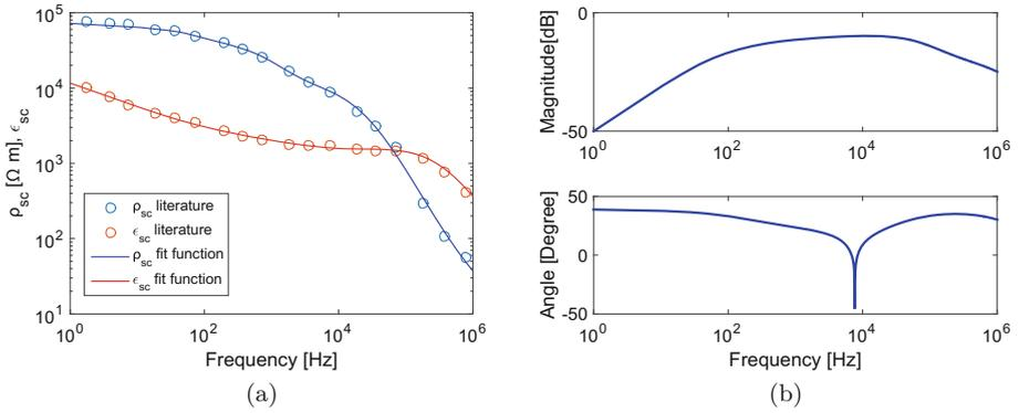
**Fig. 2.** a. The resistivity and dielectric constant of epidermal stratum corneum by [30] and the polynomial functions fitted by us on the experimental data points. b. Bode plot of the transfer function  $\frac{V_{sc}}{V}$ . (Color figure online)
