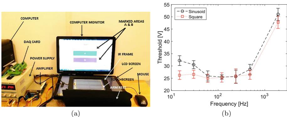
**Fig. 5.** a. Illustration of the experimental setup used in absolute threshold detection experiments. b. Absolute detection thresholds for seven fundamental frequencies and two waveforms, sinusoidal (black) and square (red), with their mean and standard deviation errorbars. (Color figure online)
