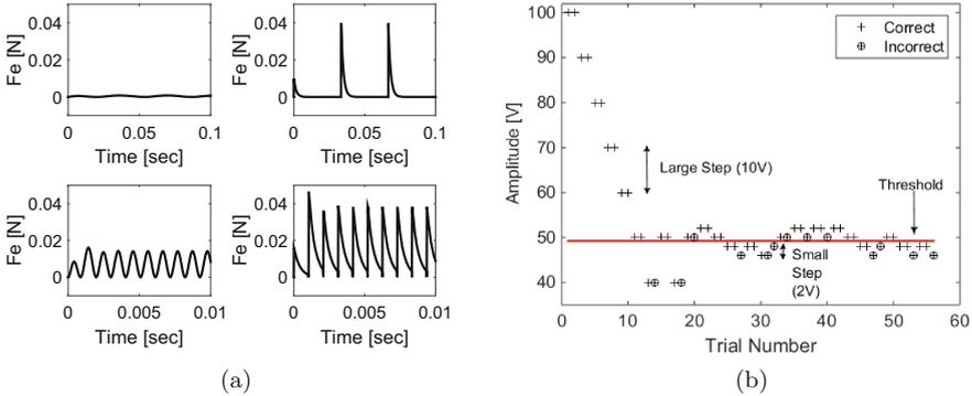
**Fig. 4.** a. The resulting electrostatic force across stratum corneum,  $F_e$ , for the four cases, calculated by Eq. 2. b. Illustration of absolute detection threshold experiment utilizing one-up/two-down adaptive staircase method. The large and small steps and the estimated threshold are marked on the figure.
